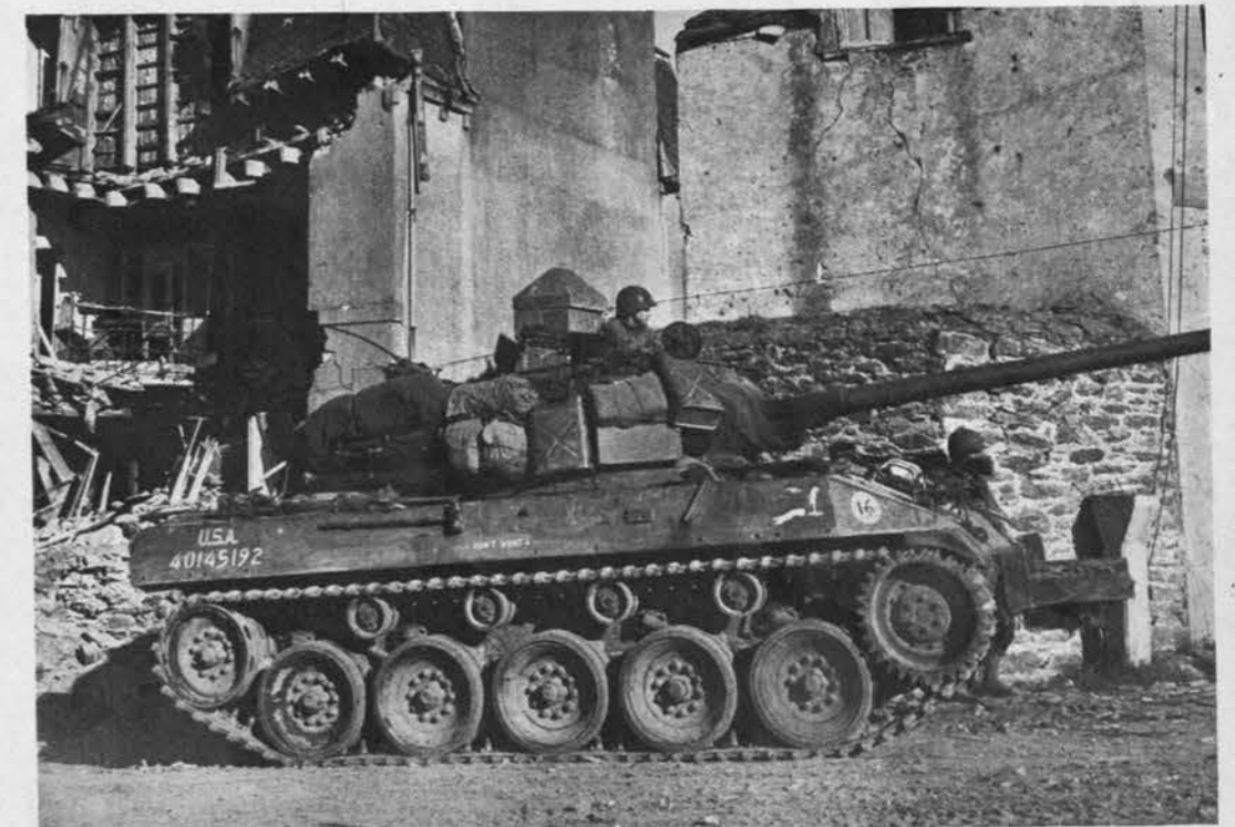
M-18 tank destroyer was first U.S. vehicle with the torsion-bar running gear used in combat. Its front sprocket, five bogies, four return rollers are also used on SP guns built on the M-24 chassis.
